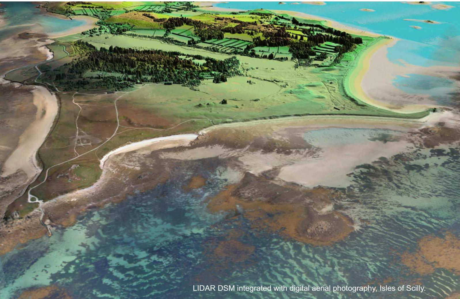
LIDAR DSM integrated with digital aerial photography, Isles of Scilly.
